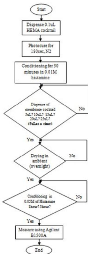
Fig.4 Procedural Flow of Membrane Deposition
