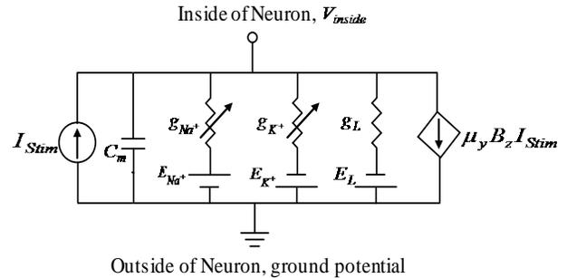
Fig.4 Expanded Equivalent Circuit Model of Neuronal membrane in Presence of Magnetic Field
