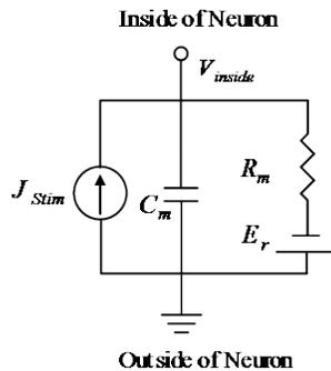
Fig.1 Equivalent circuit model of the neuronal plasma membrane characterizing the passive response of the neuron to electrical excitation in the form of a depolarizing current
