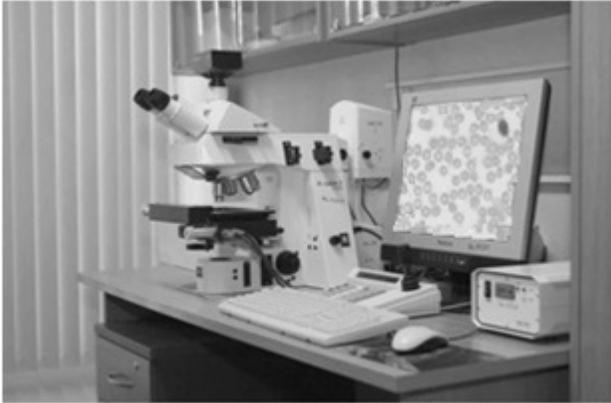
Fig.1. Computer microscope system for automatic scanning of blood smear on glass.
