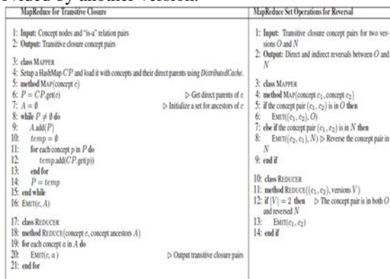
Fig.6 Left - MapReduce steps to compute transitive closure. Right - MapReduce steps to compute reversals [18]
